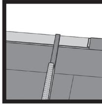
Last row (and perhaps also first row). Minimum width 50 mm. Remember distance to wall ca 10 mm. Tip! Put a distance before measuring Cut the panels lengthwise and glue the short ends.
