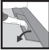
Fold the panel down in a single action movement with a slight press to the left to the short end of the previous panel.
