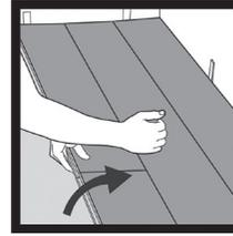
Separate the whole row by carefully lifting up and slightly knocking just above the joint.
