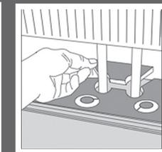
Installation at radiators. Drill the holes 20 mm larger than the diameter of the pipes
