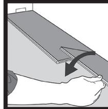
Fold the panel down in a single action movement. During the fold down, make sure the panels are tight against each other.
