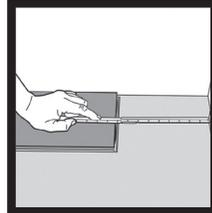
At the end of the first row, put a distance  $\approx 10$  mm, to the wall and measure the length of the last plank to fit.
