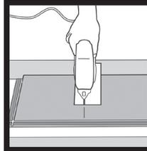
Cut with a jig saw - hardwood turned down or with a hand saw with the hardwood visible.
