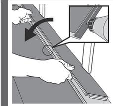
Cut off the locking element with a chisel, push the planks horizontally together. If necessary, place some distances between the last panel and the wall to keep the planks together during the curing time of the glue
