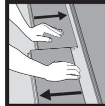
Disassemble the panels by sliding horizontally.
